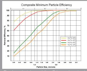
The above chart shows relative efficiency values at various particle sizes when tested in accordance with ASHRAE Standard 52.2-2007. When tested in accordance with Appendix J of that Standard the Hi-Flo maintains these efficiency values throughout the life of the filter.
